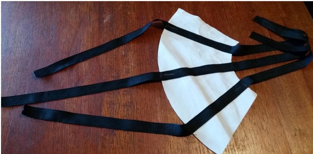
Initially I tried making the cones from rip stop nylon. However, it was too flexible and the cones crumpled instead of opening out into the cone shape. The best way to cut the sail cloth is with a hot knife as it seals the edges. I used an electric soldering iron with the tip filed to give an edge at 45 degrees to the handle. Let me know if you want to try making your own Jordan series drogue and I'll send you a copy of the template I made for cutting out the sail cloth.
