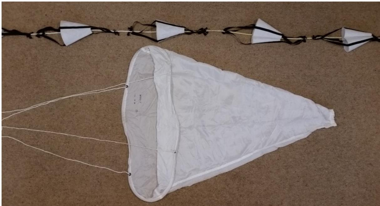
Jordan's experiments revealed one of the problems with large, single drogues. *"The tests clearly showed that a drogue deployed from the stern can pull the boat through the breaking wave crest without capsize. However, if the towline has excessive slack at time of the wave strike, the boat can be capsized before the drogue pulls."* There are also reports of drogues inverting and being
